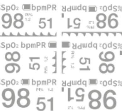
Press the power button continuously during the monitoring process. The data monitored and display method will be displayed cyclically on the OLED screen in two different ways (large fonts and plethysmograph) and in four directions, as shown in the illustration.
