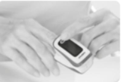
Insert a finger fully into the oximeter's measuring sections. Keep the surface of the nail pointing upwards and release the clip. Press the power button to switch on this interface as well as the upper and lower limits of the "PR" pulse rate alarm.
